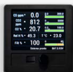
SAM sensors CO + CO 2 + H 2 O. Available in version with VOC
